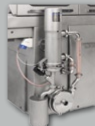
The self-cleaning protein filter FM 80 and high performance centrifugal pump.
