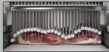
Sectionally-divided stripper feet prevent the product from moving when the needles are retracted.
