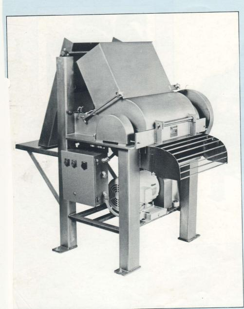
The ROTOCLAW II reduces hard frozen blocks with no aggravating noise. Its slow speed rotor produces chunks without destroying the texture of the product.
