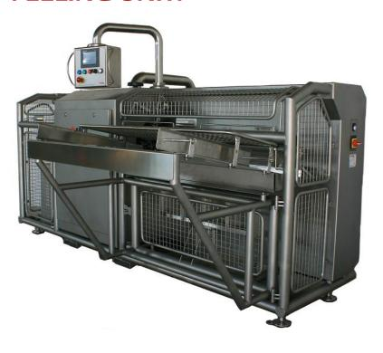
The peeling unit is composed by several areas, an exclusive area where the gut is blown, an area where the ends, the staple and the cord are removed and an area where the gut is extracted.
