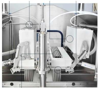
**Needle register** Needle configuration can be optimally selected for the product.
