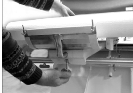
INSTALL & ADJUST PRESSURE PLATE
