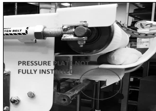
ENSURE PLATE IS FULLY INSTALLED
