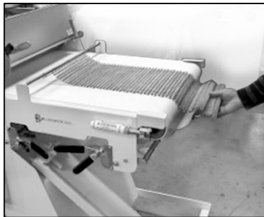
DISCONNECT MACHINE FROM POWER SOURCE. LIFT OFF CURLING CHAIN
