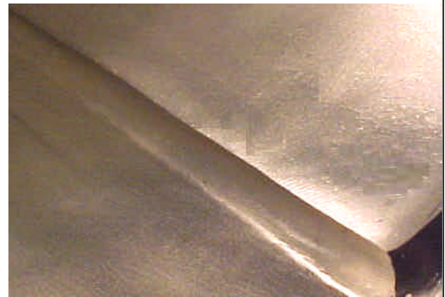
Detail of rebuilt spin ridge, note the sharp corner.
