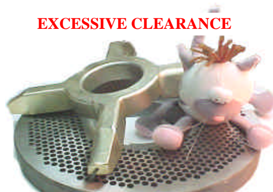
Check the knifeholder for flatness after the inserts are installed, it should not rock. Knifeholders that rock do not work. If there is any clearance, a few thousandths of an inch, .005 or less it may be at the center of the knifeholder. Clearance at the outside will cause the grinder to fail to function.
