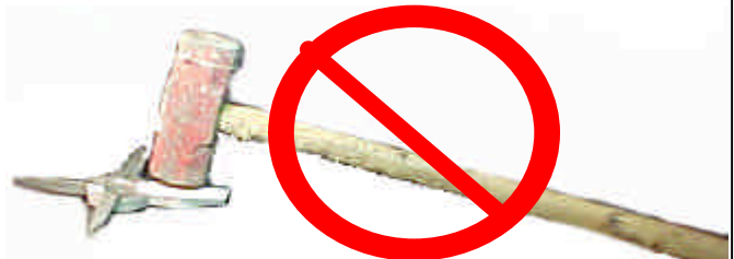
Use a soft mallet, a block of soft wood or soft plastic to tap the inserts in place.
