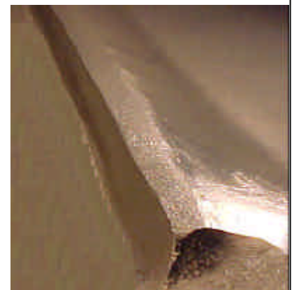
Detail of additional flute, note the sharp corner.
