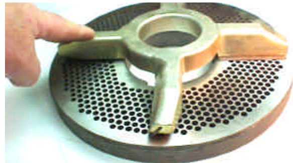
Check the knifeholder for flatness after the inserts are installed, it should not rock. Knifeholders that rock do not work. If there is any clearance, a few thousandths of an inch, .005 or less it may be at the center of the knifeholder. Clearance at the outside will cause the grinder to fail to function.
