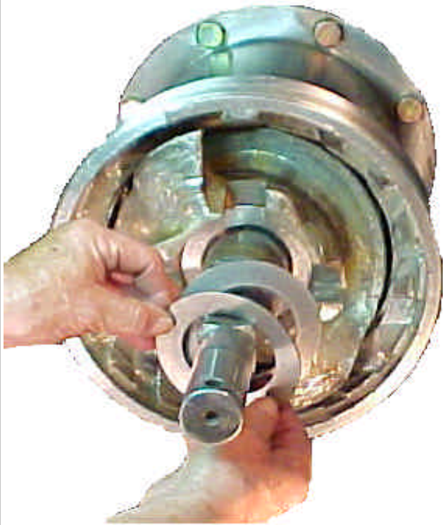
Step 7 continued, installing #10035 springs.
