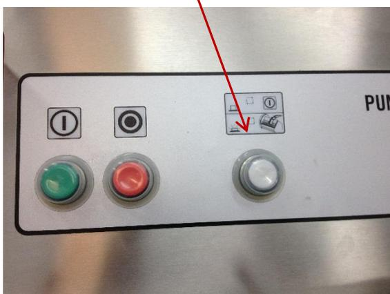
6. Close the chamber lid and drive the gripper forward with the **forward jog button** until it reaches the forward stop, ensure the DVS system does not engage. If it does, jog the gripper back with the **reverse jog button** approximately 1mm.
